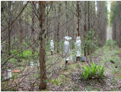
Monitoring sapflow in six year old E. nitens trees in the Florentine valley (photo: Maria Ottenschlaeger)
