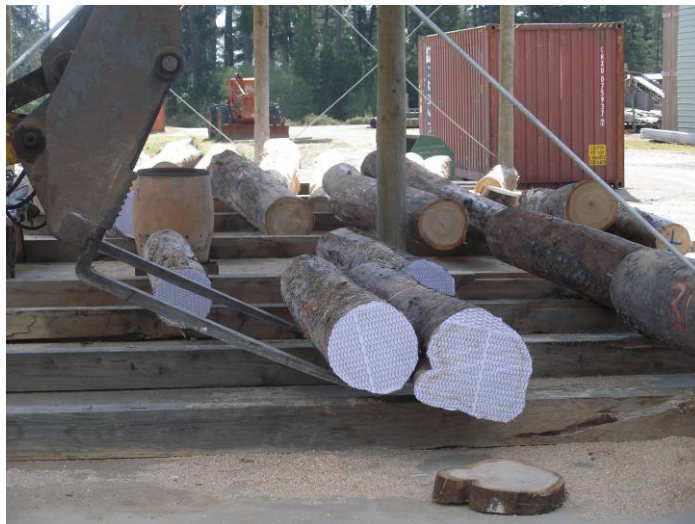
Figure 1. 2.7m-long sawlogs following cross-cutting of bush logs at Creswick Timber Training Centre, with log-end templates affixed prior to sawing
