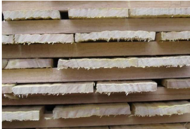
Figure 9. Board cross-sections after drying and prior to reconditioning (displaying ‘washboarding’)
