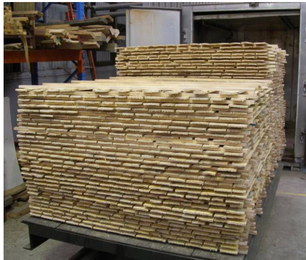
Figure 4. Two stacks of boards, outside the drying kiln, prior to reconditioning
