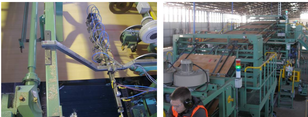
Figure 7. Billet identity of individual veneer sheets maintained using paint colour combinations applied by paint nozzles
