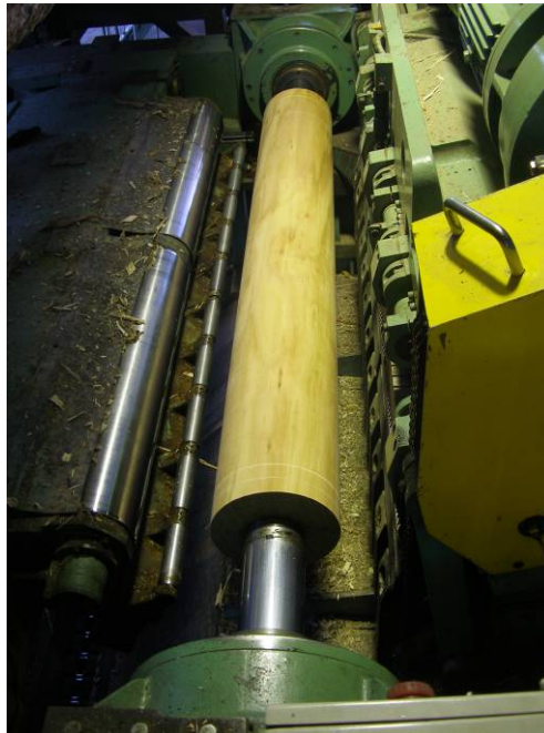
Figure 6. Lathe, with partly peeled E. nitens billet
